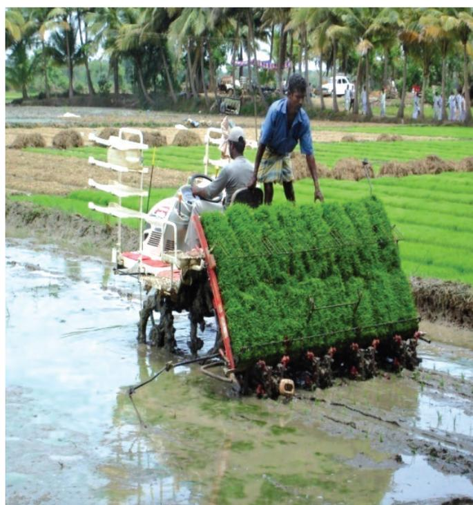
**Fig. 4. Self propelled riding type transplanter**
