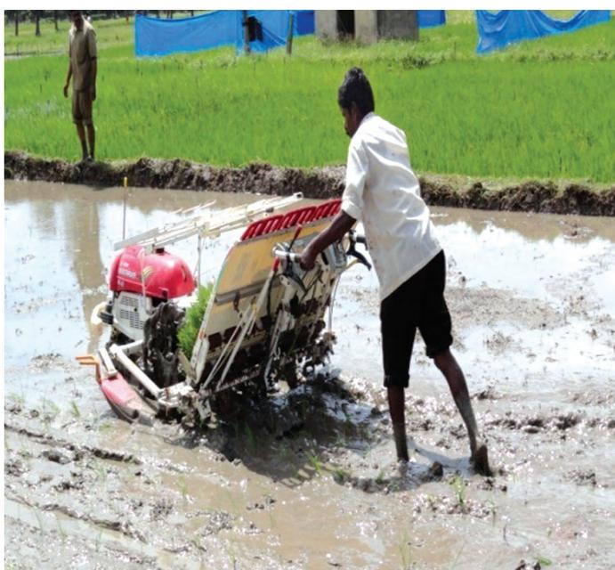
**Fig. 3. Self propelled walk behind type transplanter**
