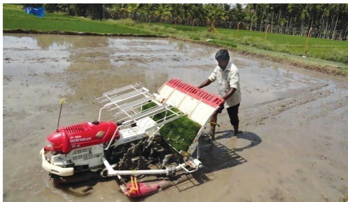
Fig. 1. Self propelled walk behind rice transplanter (kukje) in operation
